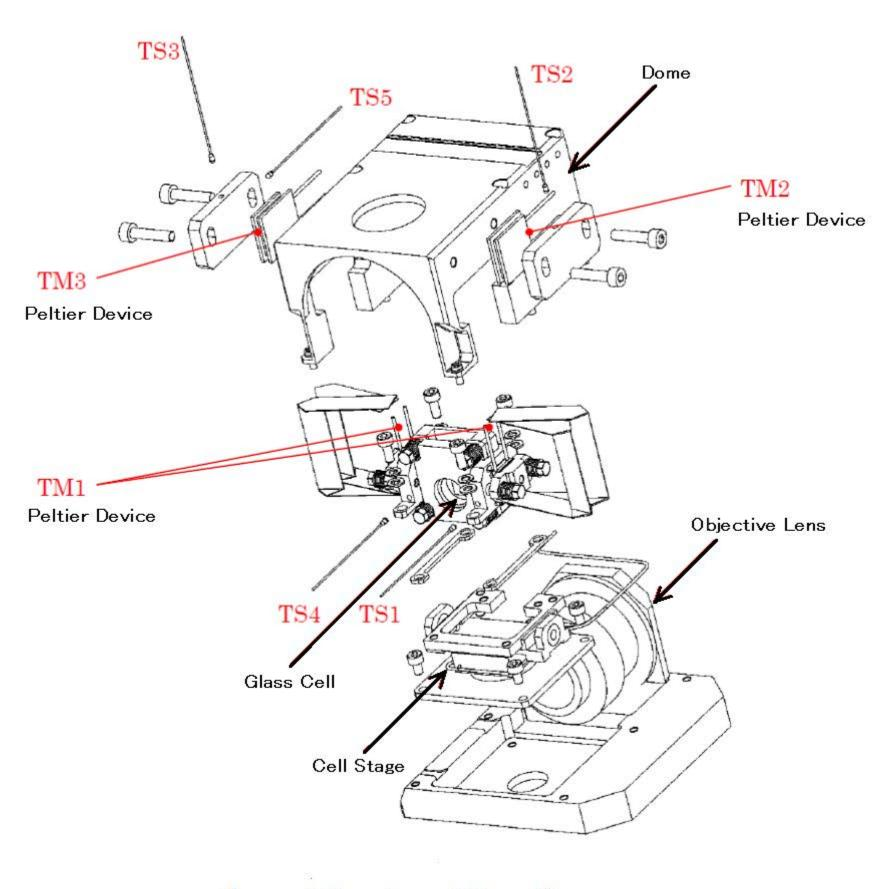
General Drawing of Nano Step (Specimen Cell Unit)
