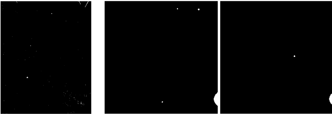
Figure 5.10.12: Mask files for NIR, MIR-S, and MIR-L (from left to right). Outlier pixels to be masked have a value of 0 (white) and others 1 (black).
