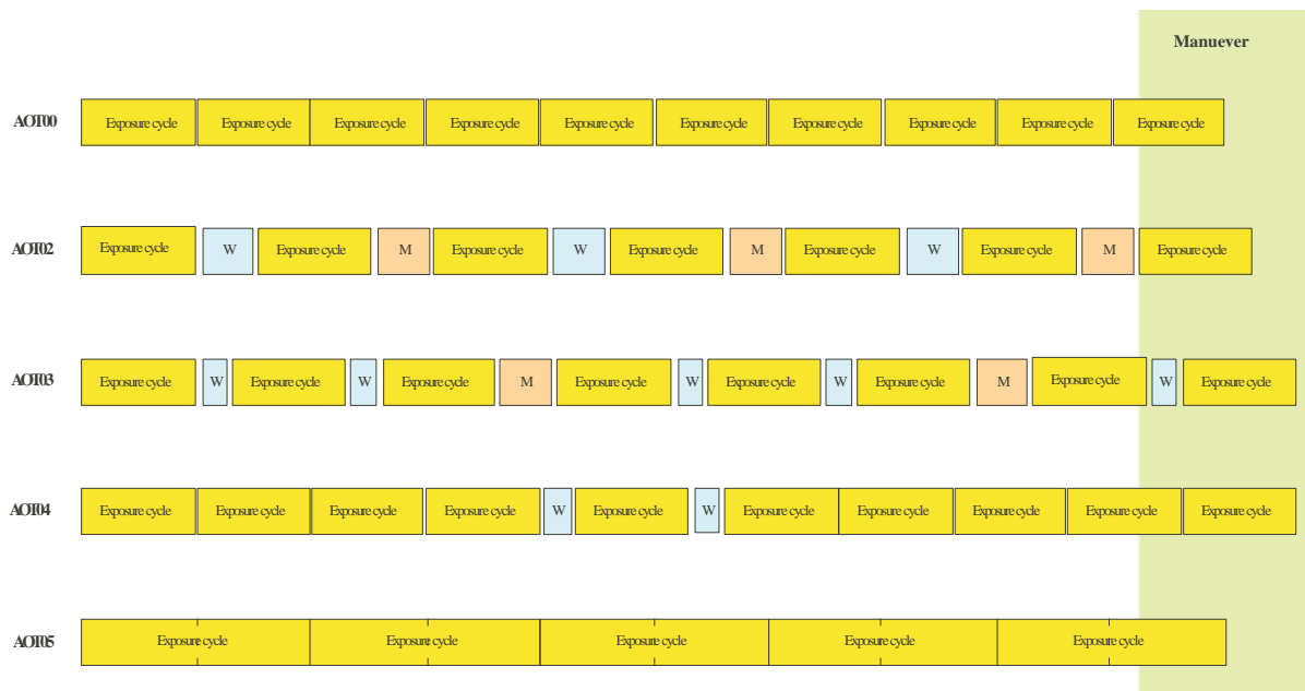
Figure 2.2.6: Observation sequences of the AOT IRC00, 02, 03, 04 and 05. Yellow boxes labeled as “Exposure cycle” indicate exposure frames. Orange boxes with “M” are Micro-Scan (i.e. dithering) operations including stabilization, and light-blue boxes with “W” are Filter Wheel rotations. Dead time for a Filter Wheel change depends on the relative position of the elements. The Green area on the right side is the extra observation time which is not guaranteed.
