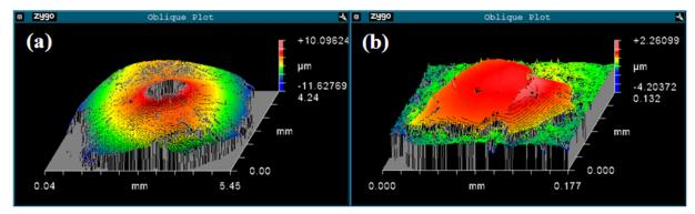
Surface profiles of the 6mm epoxy disk containing the Itokawa particle RA-QD02-0010 (a) and the particle located at the center of the disk (b). The surface profile data were obtained by a ZYGO white light profilometer at the Material Science Center (UW-Madison) before SIMS analyses. In panel a, surface profile data of the central area are lacking, because Au-coating was removed and surface was dim.
