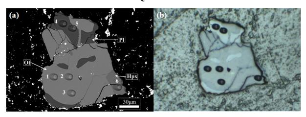
Images of the Itokawa particle RA-QD02-0010 after SIMS analyses; (a) back scattered electron image (Nakashima et al. 2013, EPSL) and (b) optical microscope image. In panel a, numbers near the SIMS pits in the image indicate spot numbers of SIMS analysis, which correspond to spot numbers in a table shown below. Abbreviations: Ol, olivine; Pl, plagioclase; Hpx, high-Ca pyroxene. White materials around the particle are remnant of Au-coating.
