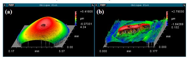
Surface profiles of the 6mm epoxy disk containing the Itokawa particle RA-QD02-0014 (a) and the particle located at the center of the disk (b). The surface profile data were obtained by a ZYGO white light profilement at the Material Science Center (UW-Madison) before SIMS analyses.
