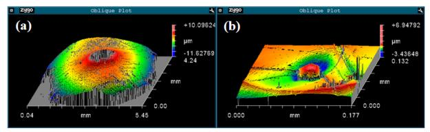
Surface profiles of the 6mm epoxy disk containing the Itokawa particle RA-QD02-0017 (a) and the particle located at the center of the disk (b). The surface profile data were obtained by a ZYGO white light profilometer at the Material Science Center (UW-Madison) before SIMS analyses. In panel a, surface profile data of the central area are lacking, because Au-coating was removed and surface was dim.
