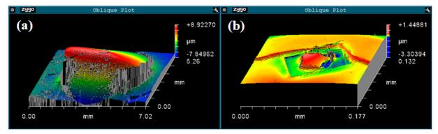
Surface profiles of the 6mm epoxy disk containing the Itokawa particle RA-QD02-0196 (a) and the particle located at the center of the disk (b). The surface profile data were obtained by a ZYGO white light profilometer at the Material Science Center (UW-Madison) before SIMS analyses. In panel a, surface profile data are partly lacking, where there are scratches and surface was dim.
