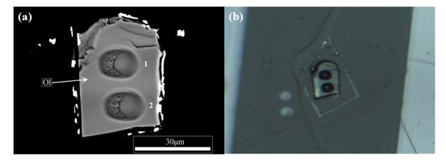
Images of the Itokawa particle RA-QD02-0196 after SIMS analyses; (a) back scattered electron image (Nakashima et al. 2013, EPSL) and (b) optical microscope image. In panel a, numbers near the SIMS pits in the image indicate spot numbers of SIMS analysis, which correspond to spot numbers in a table shown below. Abbreviations: Ol, olivine. White materials around the particle are remnant of Au-coating.
